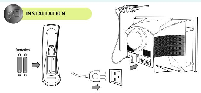
Open remote control battery compartment (at the rear) and insert two 1.5V type AAA batteries. Warning: be careful to respect battery polarities.
